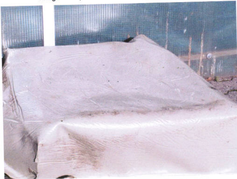
Image 2: Bottom side without root ingress
