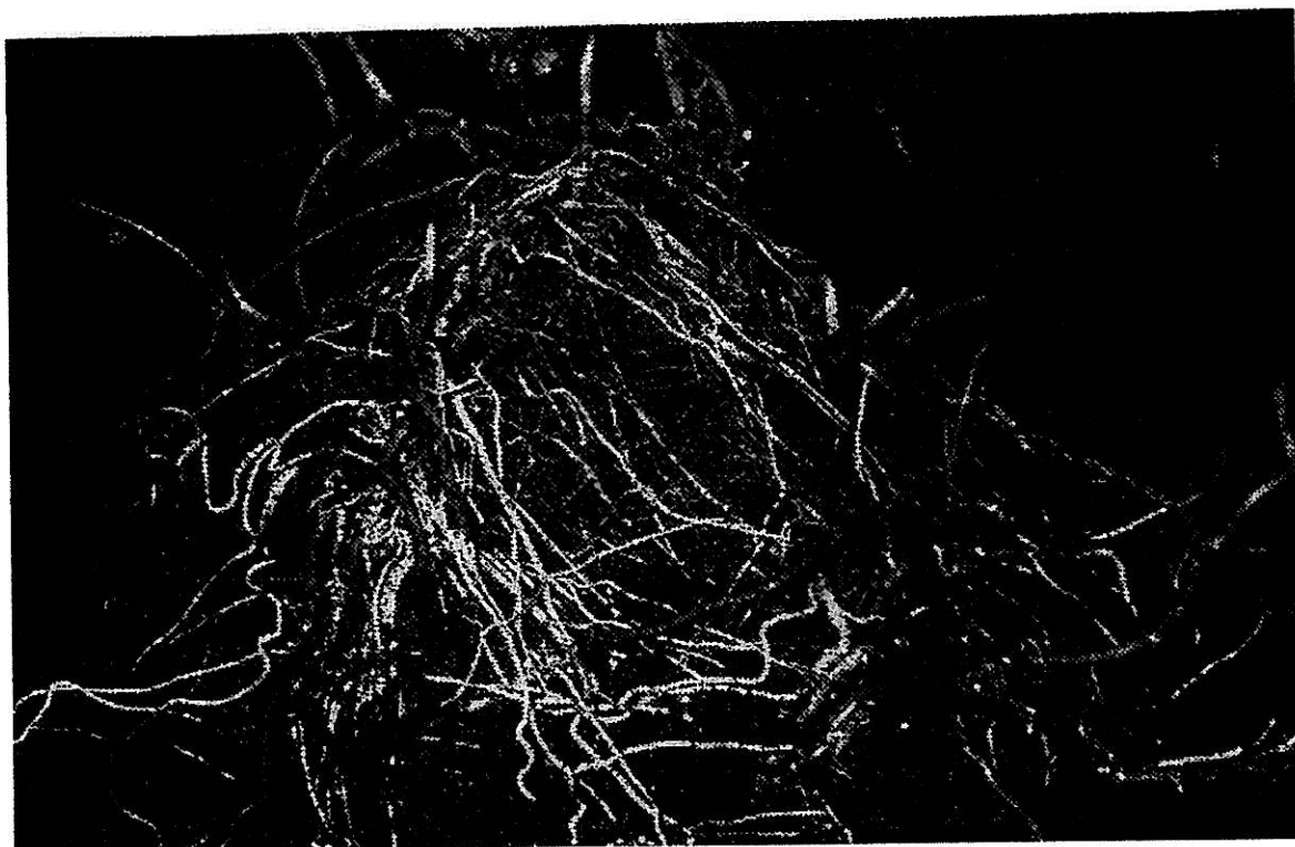
Fig. 4. View of the underside of compost completely infiltrated by roots taken from a test container lined with KEMPEROL® V 210
