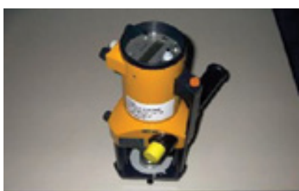
Measuring instrument for testing the tensile strength (adhesion)
